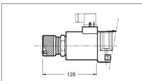
When the set screw is screwed and its point is aligned with the edge of the knob, tighten the knob till it touches the spool: in this position the override is not engaged and the valve is de-energized. After adjusting the override, tighten the set screw in order to avoid the knob loosing.
