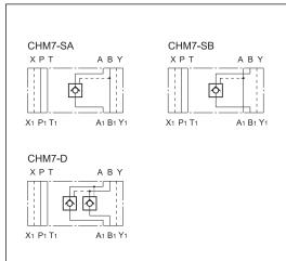
CHM7 PILOT OPERATED CHECK VALVE SERIES 11
