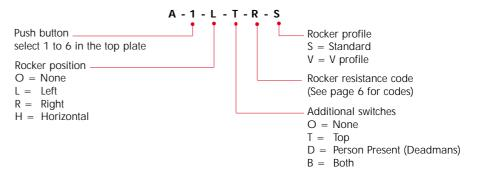
Note: When ordering a handle fitted with a rocker, two profiles can be supplied (S = standard profile; V = v profile) please specify style when ordering.
