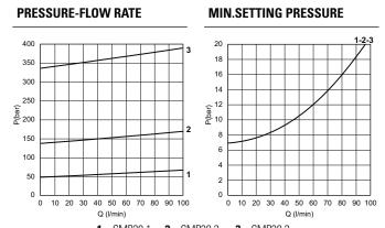
$\textbf{1} = \text{CMP30.1...} \cdot \textbf{2} = \text{CMP30.2...} \cdot \textbf{3} = \text{CMP30.3..}$  Fluid used: mineral based oil with viscosity 46 mm²/s at 40°C.
