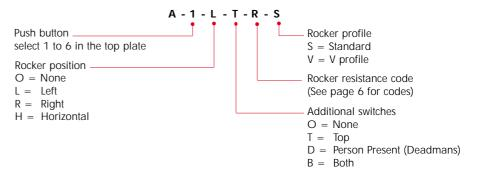
Note: When ordering a handle fitted with a rocker, two profiles can be supplied (S = standard profile; V = v profile) please specify style when ordering.
