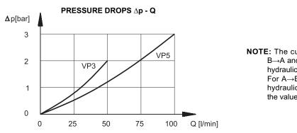
**NOTE:** The curves shown in the graph refer to B→A and A→B flow with the valve released hydraulically.
